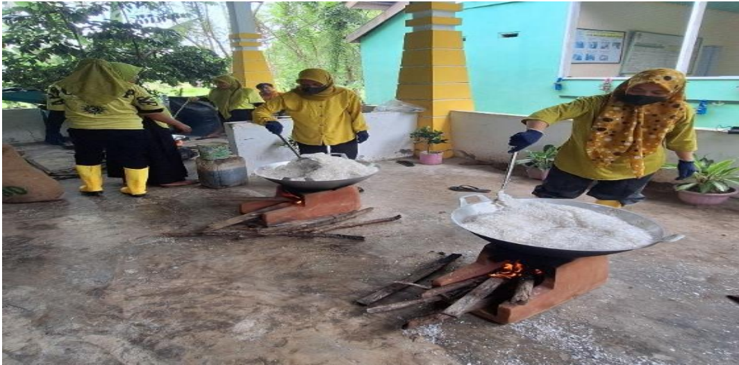
Gambar 6. Proses Pelelehan Limbah Plastik Cacah
