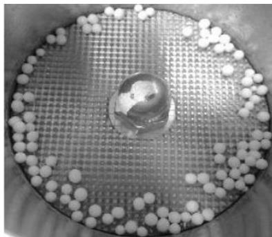
Figure 3. The pellets in the spheroniser after 8 minutes of rotation [17].
