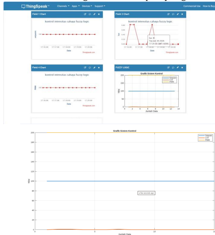
Gambar 5. Grafik Monitoring ThingSpeak Kondisi Sensor Tertutup
